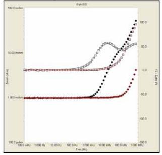
The black and grey data were recorded using the Reference 600's standard cell cable. Its alligator clips were attached to the pins on the resistor/header assembly. The red and pink data were recorded with a Low Impedance cable for the Reference 600 connected as described above.
