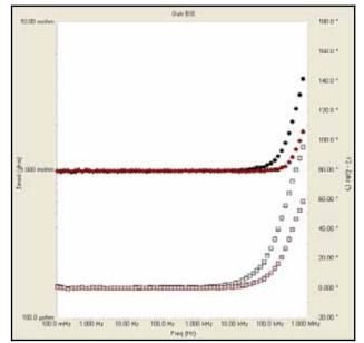
Figure 5 shows the resistor's spectrum before (in black and grey) and after (in red and pink) a series subtraction of the surrogate's spectrum.
